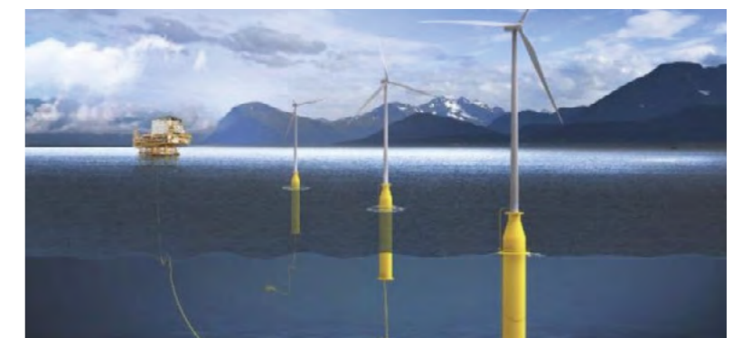
Foundation for a floating wind turbine
