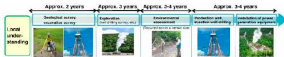
General flow of geothermal development (model case of 30,000 kW power output)
