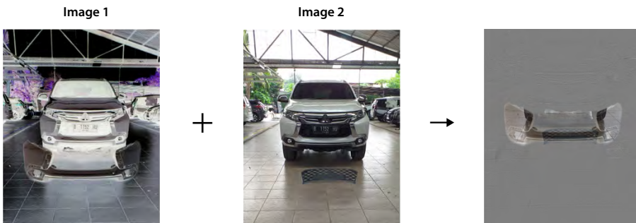
Example of fraud detection in accident images: An analysis by AI indicated that images 1 and 2 were derived from the same image and that the front part in each image has been deliberately doctored to disguise it as being repaired.
